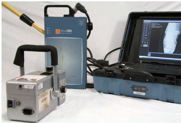
In this photo, the DR unit is set up. Note the portable computer on the right showing the image that has just been taken. The image plate is the blue rectangle in front of the small portable x-ray machine at the bottom left - this captures the x-rays and transmits the information through the cable to the computer.
